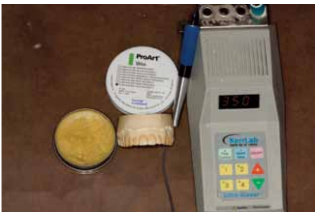
Figure 4: View of wax and waxer used for application on the stone model.
