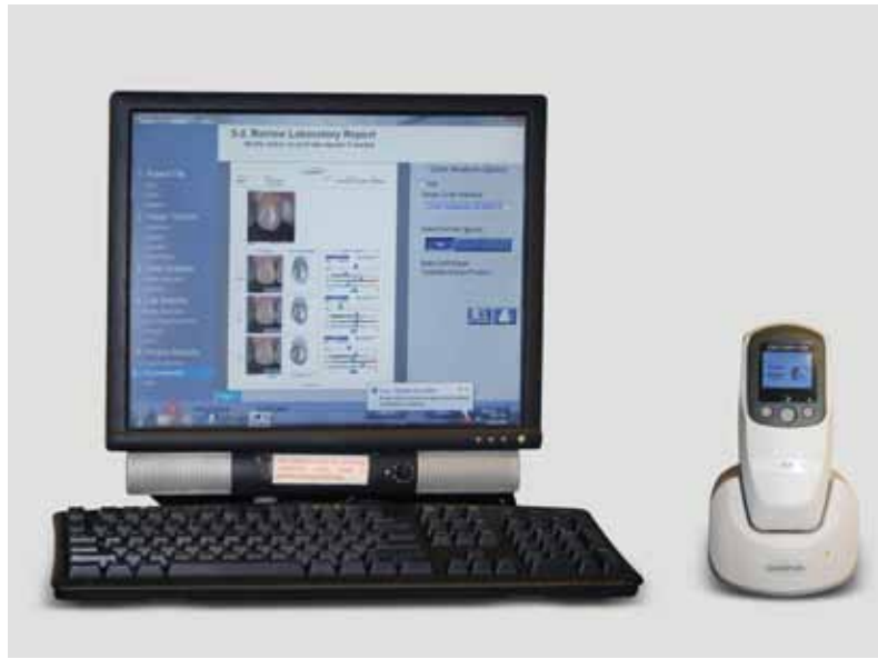
Figure 3: A Crystaleye Spectrophotometer was used to digitally color map the right central incisor. The information was transferred to computer software, analyzed, and used to assist in selecting composite materials with the correct color and translucency.
