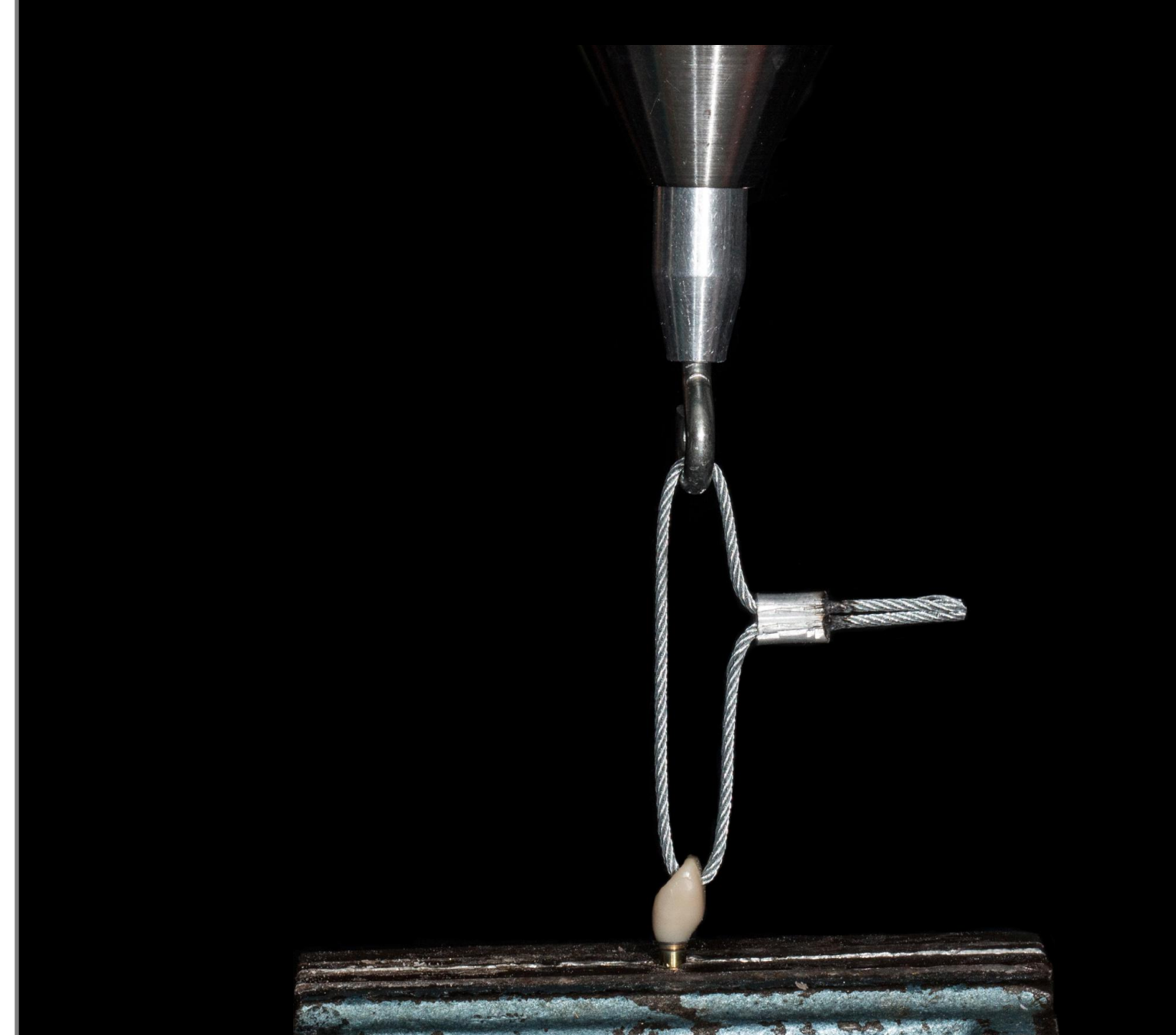
Fig 7. Pull-Out Device for crown retention testing
